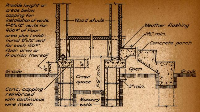
Concrete capping placed on kraft paper impregnated with coal tar pitch. Wood sills bedded and anchor bolts pointed with coal tar pitch.
