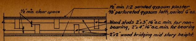
No connection between study on one side of partition to study on other side shall be made, except at floor and at ceiling.
