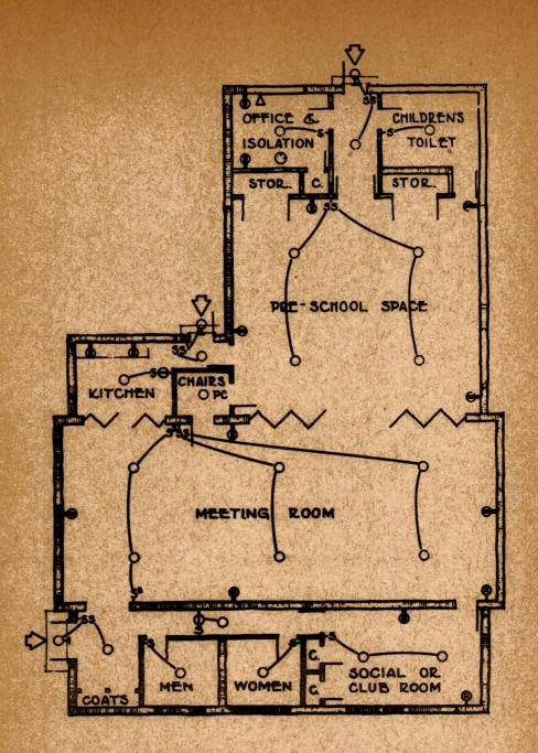
THIS LAYOUT IS TO INDICATE THE ARRANGEMENT OF ELECTRICAL WORK ONLY FOR THE VARIOUS SPACES. THIS PLAN IS NOT NECESSARILY APPLICABLE FOR BUILDING DESIGN.
