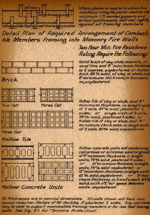
Where plaster is required to obtain fire resistance rating, the plaster shall be 1/2" minimum 1:3 sanded gypsum and extend continuously past and tightly against all froming members
