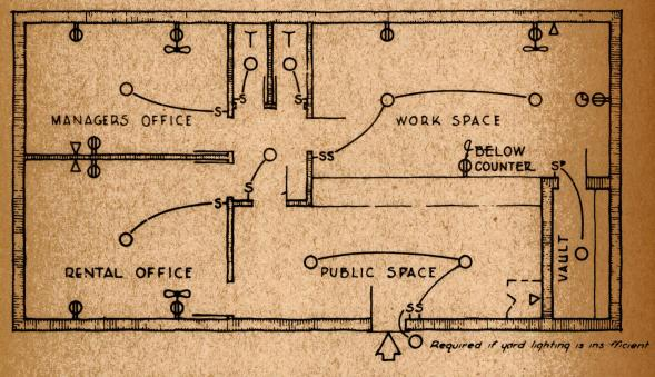
THIS LAYOUT IS TO INDICATE THE ARRANGEMENT OF ELECTRICAL WORK ONLY FOR THE VARIOUS SPACES THIS PLAN IS NOT NECESSARILY APPLICABLE FOR BUILDING DESIGN
