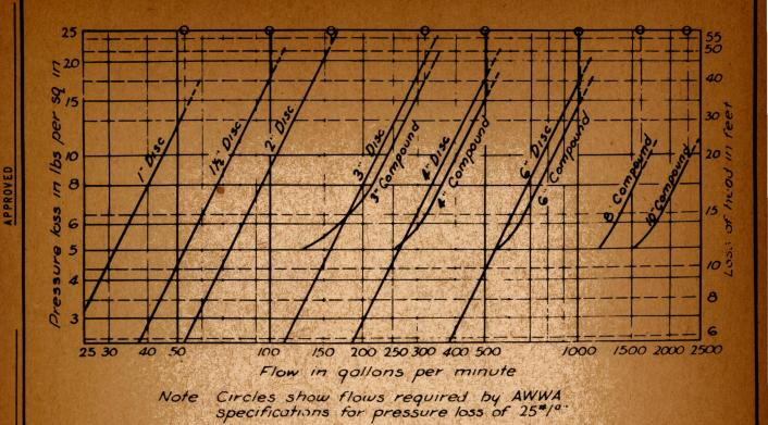
DATE APPROX. PRESSURE LOSSES THRU COLD WATER METERS FPHA
