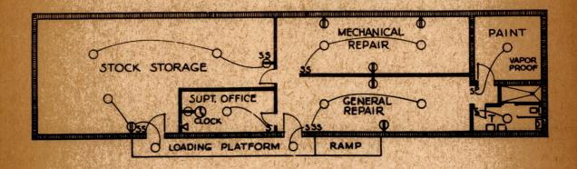
THIS LAYOUT IS TO INDICATE THE ARRANGEMENT OF ELECTRICAL WORK ONLY FOR THE VARIOUS SPACES THIS PLAN IS NOT NECESSARILY APPLICABLE FOR BUILDING DESIGN.
