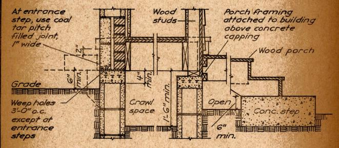
Concrete cappings to be continuous of poured concrete of 2000 lb. strengthdry consistency. Interior masonry piers and walls to be similarly capped.
