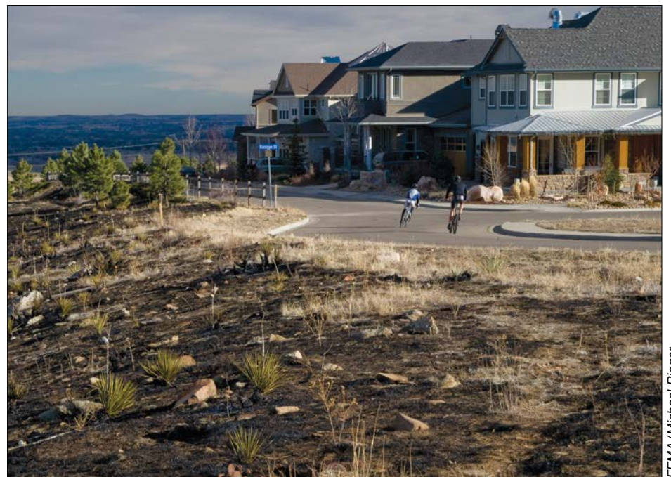
This Colorado neighborhood’s outer road, which doubles as a fire barrier, protected these homes from wildfires in 2009.
