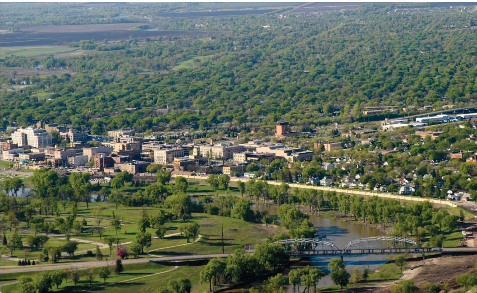
The centerpiece of Grand Forks' new flood protection system is the Greenway, parkland between the river and the new dike system that can be safely flooded during periods of high water and used as recreation space at other times.
